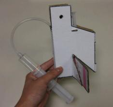
Now you should have a frame housing a syringe that will be responsible for lifting and dropping a mechanical arm, which you will be able to control using the larger syringe.
